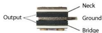
Straight switch Bottom view, lugs bent:
